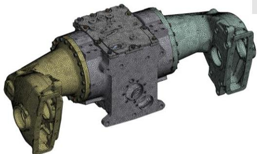
Mesh of a tractor axle by Ansys Mechanical™ software. assemblies require modeling contact between parts as well as specific interfaces, such as gaskets.
