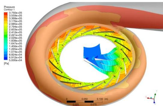
Multi-frequency harmonic analysis by Ansys CFX® provides fast solutions to challenging transient periodic flow cases such as simulating fans under inlet and outlet disturbances or modeling the asymmetric flow in radial compressors or turbines.
