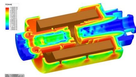
Magnetic flux distribution on magnetic actuator by Ansys Maxwell®. This type of analysis helps in predicting the characteristics of solenoid as force vs position in magnetostatics solver or position vs time in transient solver.
