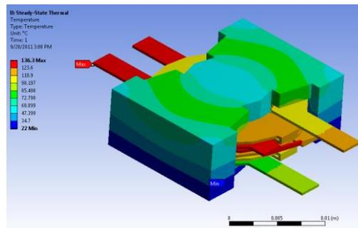
Temperature Profile within Electronic Transformer – Power loss of a transformer solved with Maxwell, then transferred to Ansys Mechanical to calculate thermal distribution
